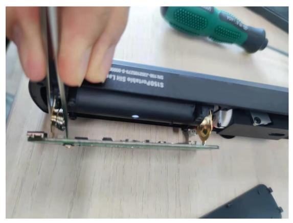
Hold the spring with tweezers and pass it out from the other side. (Note that at the same time also pass through the copper sheet at the other end)
